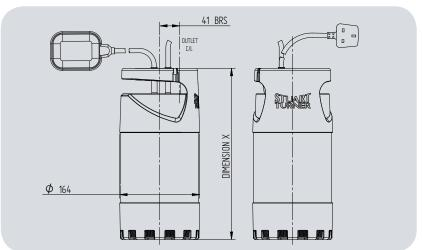
The Diver pumps are supplied complete with hose union, suitable for 25 mm (1") bore hose.
